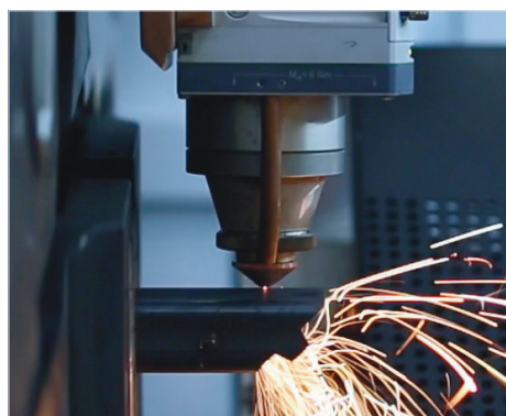
■ Performs precision and rapid cutting operations thanks to its structure resistant against higher acceleration and high pressure. (S)
